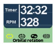
Orbital rotation - clockwise classic platform motion mode with adjustable speed and time parameters.
