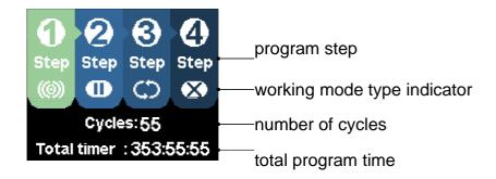
You can set the number of repeat cycles on the bottom line of the programming menu. Ranges are from 1 to 99, or continuos mode can be used. Create a custom cycle program by adding four steps and a number of program repeat cycles as required.
