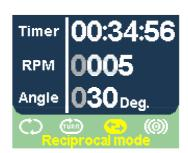
Reciprocal mode - provides changing direction motion with the choice of rotation angle of the platform, at a predetermined RPM and operating time.
