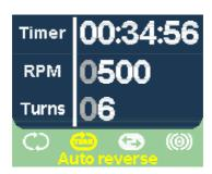
Auto reverse mode - platform orbital motion mode with set and equal numbers of clockwise and counter-clockwise turns.
