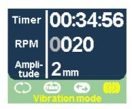
Vibration mode - reciprocating type of movement of the platform imitating shake.
