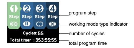
You can set the number of repeat cycles on the bottom line of the programming menu. Ranges are from 1 to 99, or continuos mode can be used. Create a custom cycle program by adding four steps and a number of program repeat cycles as required.
