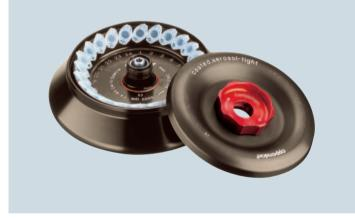
Aerosol-tight rotor for  $24 \times 1.5/2$  mL tubes with PTFE-coating for high chemical resistance. Provides speed up to  $21,130 \times g/$ 15,000 rpm (FA-45-24-11-Special; Order no. 5424 700.004).
