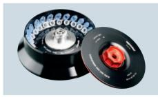
**Eppendorf Kit rotor** for 24 × spin columns and 1.5/2.0 mL tubes. Designed with an extra high rim to support open tube lids during centrifugation. Spins at max. 19,090 × q/13,200 rpm (FA-45-24-11-Kit\*; Order no. 5427 752.005).
