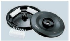
8 × PCR strip rotor with removal adapters that can be used as a pipetting rack; maximum speed is  $13,543 \times g/11,800$  rpm (F-45-64-5-PCR; Order no. 5427 714.006, includes adapters).
