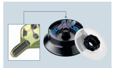
**Eppendorf Kit rotor**<sup>®</sup> **for 18 × spin columns and 1.5/2.0 mL tubes** with speed up to  $18,111 \times g/15,000$  rpm. This rotor is designed with an extended rim that protects tube caps from shearing off (FA-45-18-11-Kit; Order no. 5424 706.002).
