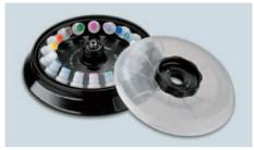
18-place rotor for Cryovials® and HPLC tubes. Speed up to  $8,324 \times g/8,900$  rpm (F-45-18-17-Cryo; Order no. 5427 705.007 incl. cryo adapters). Additional adapters: HPLC vials, pk/18; Order no. 5427 708.006
