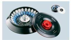
**Rotor for 48 × 1.5/2.0 mL tubes** spins up to  $18,210 \times g/12,700$  rpm (FA-45-48-11\*/\*\*\*\*; Order no. 54277 540.081). Also available with basic plastic lid (F-45-48-11\*\*\*\*; Order no. 54277 550.041).
