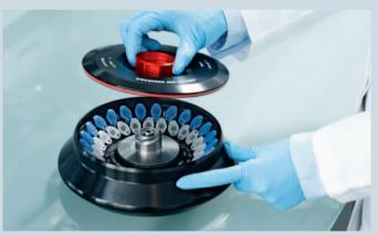
**Eppendorf QuickLock® rotors** Our aerosol-tight Eppendorf QuickLock rotors close with only 1/4 of a turn. This not only saves you time but also takes repetitive stress off your wrist.
