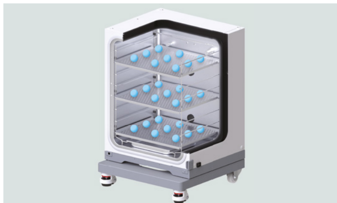
Position of the 27 sensors to verify equal temperatures at different locations.
