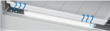
Natural Evaporation of Condensate • Interior water is drained through a small hole into a stainless steel catch box. Condensate water is evaporated by warm air flow
