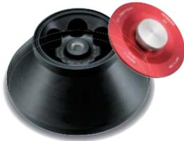
The R21A2 rotor is designed for 30ml x 6 tubes and has 40° tube cavity angle. It is suitable for pelleting. 40SS tube and 40Ti tube (for ultracentrifuge) can be used.
