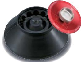
The R22A6 rotor is designed for 10ml x 12 tubes and has 45° tube cavity angle. It is suitable for pelleting. 12SS tube and 12 Ti tube (for ultracentrifuge) can be used.
