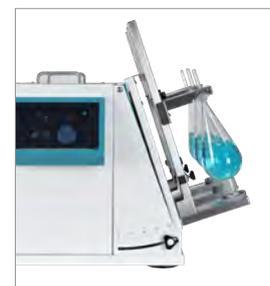
Tilt angle adjustment from 0 to 20° for maximum mixing efficiency.
