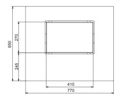
Steel Anti-Vibration Table for PA-04/H 2 900 Automatic Feeder
